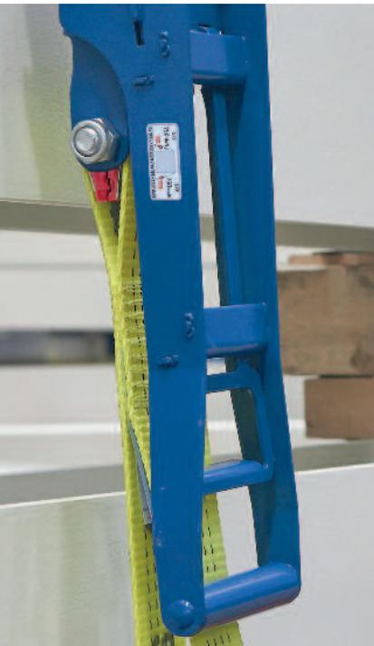
So one can describe the Tension Force Indicator (TFI) from the point of view of a user, for this tension force indicator always remains in place, because it is a "fixed component" of the lashing system.
