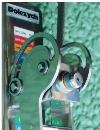
In this device a bolt becomes visible. On this bolt there are several different coloured rings. With the help of the visible rings and their colours one can read off the preload measurements in a table.
