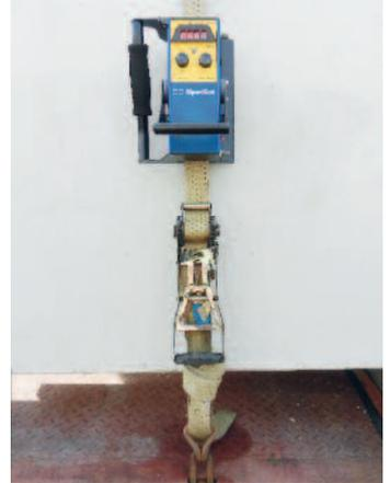
Newer devices have a digital indicator and one can accurately read the preload measurements in the display (e.g. 667 daN).
