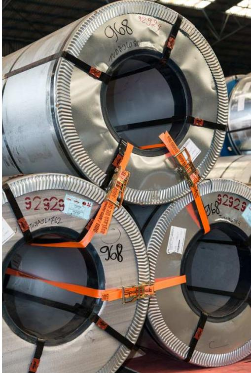
III. 1: The Dynamic Load System is also suitable for securing coils.
