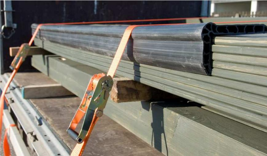
*Fig. 2: The long edge protector is very robust and warp resistant and can even bridge load gaps.*
