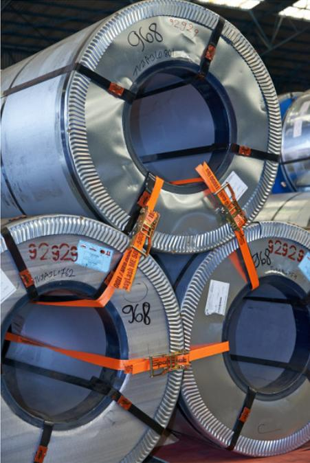
*Fig. 2: Das Dynamic Load System is especially suitable for securing coils for transport by sea.*
