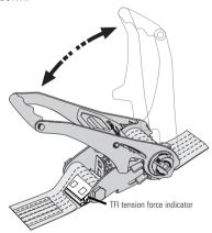
With push ratchets the belt is tensioned by pushing up and with pull ratchets (e.g. ErgoABS) by pulling down the ratchet
